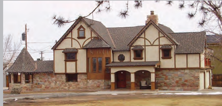
Inspired by English architecture. Most examples of this style feature ornamental half-timbering. Common elements: half-timbering, steeply-pitched roof, casement windows with mullions, clipped gables, combination hipped and gabled roof, decorative chimney detailing, bay window, heavy shingles in tile or slate, textured exterior. (Image: 6 Lakewood Heights Dr.)
