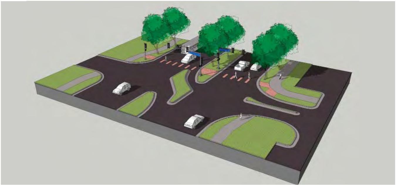
Figure 30. Union Boulevard with HAWK Signal Crossing
