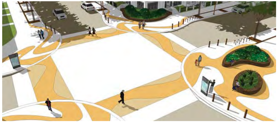
Figure 36. An example of well-designed raised crosswalks
