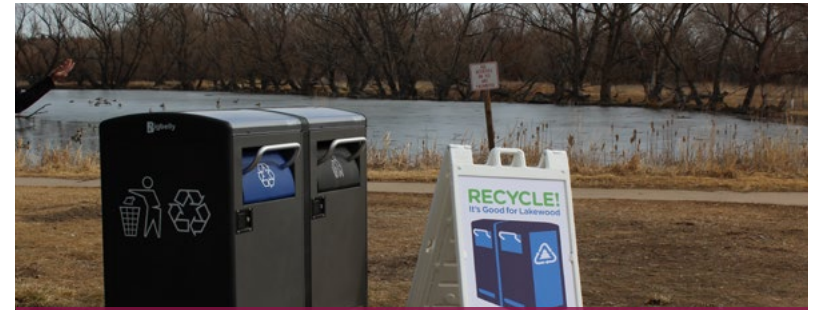
More than 100 smart recycling bins were added in Lakewood parks. These "Bigbelly" bins run on solar power and send a notification when they are full, saving staff time and tracking how much Lakewood is recycling.
