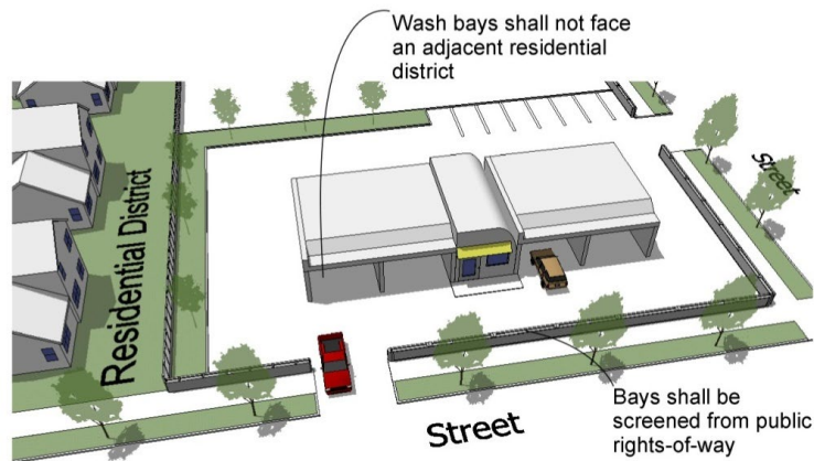
Figure 17.7.7: Car Wash Bay Location
