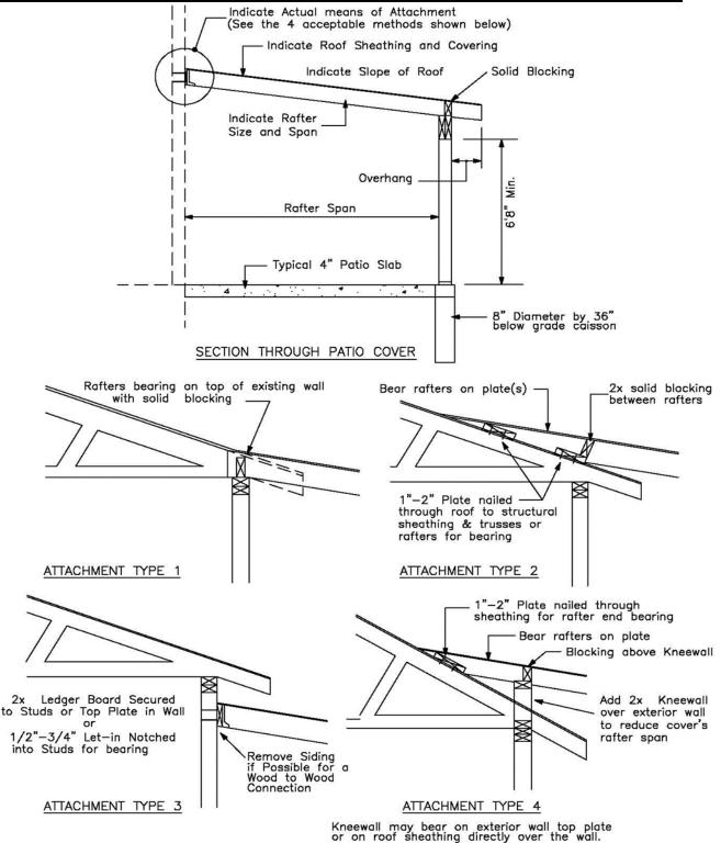
Please note that over-framing may not be installed over existing roofing materials such as asphalt shingles, bituminous membrane, EPDM membrane or similar roof finish materials. The existing roofing material must be removed to the structural sheathing to allow for flashing and proper structural connection.
